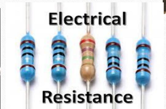
Resistance of a conductor is said to be 1 ohm if a current of 1 ampere flows through it for a potential difference of 1 volt across its end.
