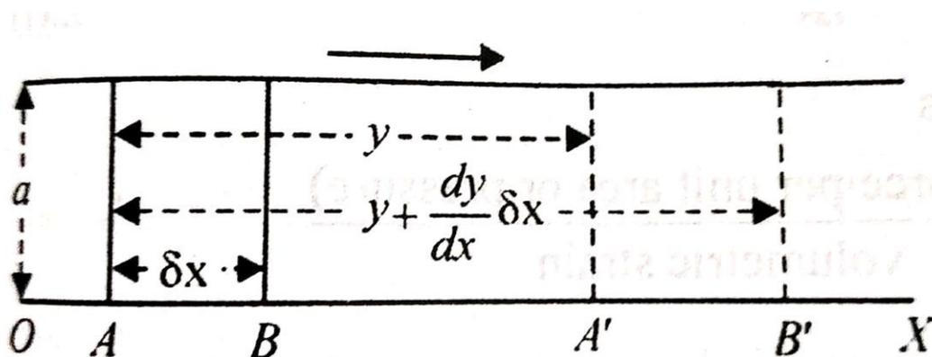
Now the displacement of the plane at  $A = AA' = y$ , the rate of change of displacement =  $\frac{dy}{dx}$
